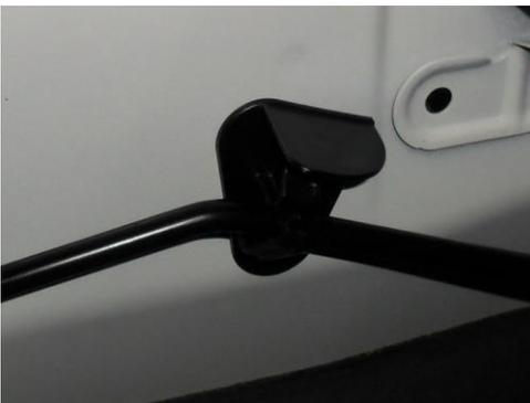
Now, swing your right hand down toward the “engine” compartment, and look for the hood support hole and insert the end of the hood support rod.
