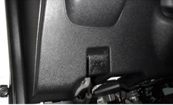
This is the hood release lever. Can you see the icon of a car with the hood up?
