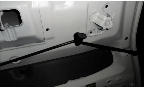
Using your right hand, grip the right end of the hood support rod, position your right elbow up high, and pull toward your elbow so that the rod pops out of the holder.
