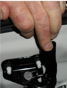
To release the safety latch, position your palm up, reach into the one inch gap, feel around for the little tab of the safety latch.
